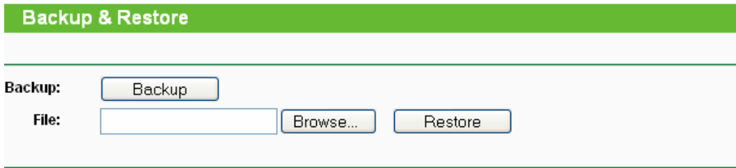
Figure 4-37 Save or Restore the Configuration
