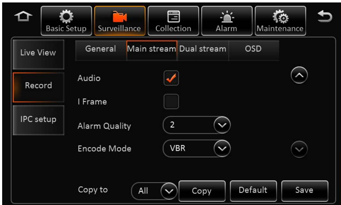
Feature 2: Added CBR (Constant Bit Rate), VBR (dynamic bit rate) coding mode, in order to accommodate the use of various camera scene.
