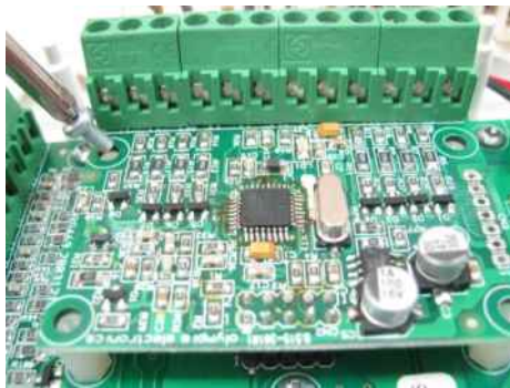
Figure 5 : installing the screws on the BS-469 board.
