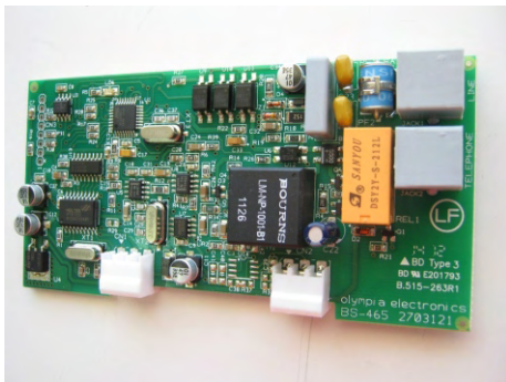
Figure 1 : View of the BS-465 circuit board .
